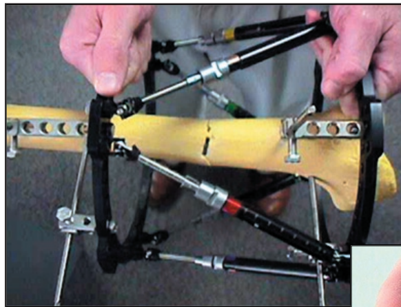
Fig. 43 Fast Fx™ struts have dual actions. With the locking sleeve released the strut length can be easily changed like a trombone slide. If six Fast Fx™ struts are used on a Spatial Frame and all locking sleeves are released the frame can be adjusted through all six degrees of freedom, analogous to an unlocked ball joint frame.
